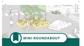
Installed using simple markings or raised islands that lower speeds at minor intersection crossings and are an ideal treatment for uncontrolled intersections.
