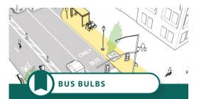
Curb extensions that align the bus stop with the parking lane, allowing buses to stop and board passengers without ever leaving the travel lane.
