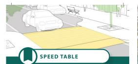
Midblock traffic calming devices that raise the entire wheelbase of a vehicle to reduce its traffic speed, often used with pinchpoints or a pedestrian walkway.
