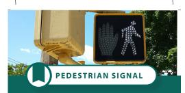
A device used at a signalized intersection with a crosswalk that informs pedestrians when to safely cross a street.
